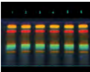
HPTLC chromatograph showing biochemical consistency of 6 batches of St. John's Wort extracts
